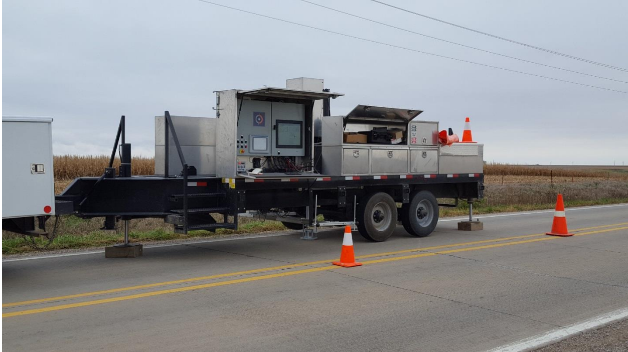
Figure 1. Automated plate load test (APLT) equipment setup on the CR V-18 project
