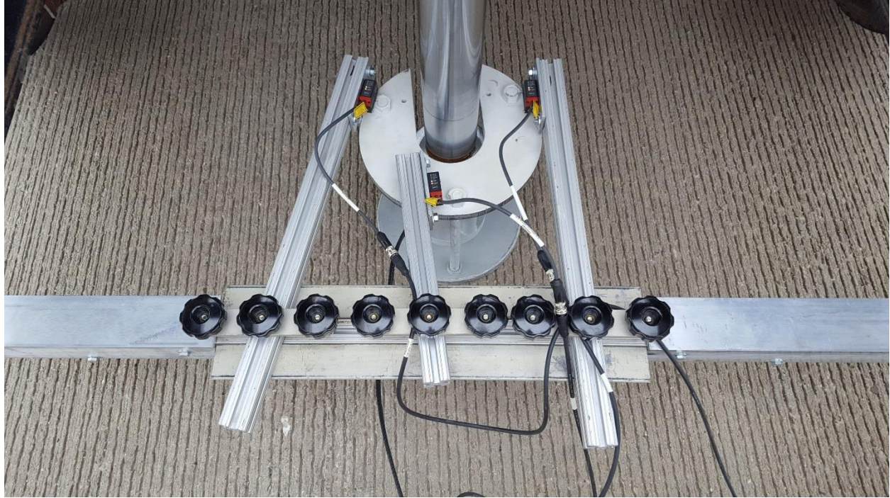
Figure 3. 12 in. diameter plate setup with reference beam for plate deflection measurements
