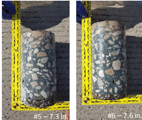
Thicknesses noted are thickness of PCC + fabric
