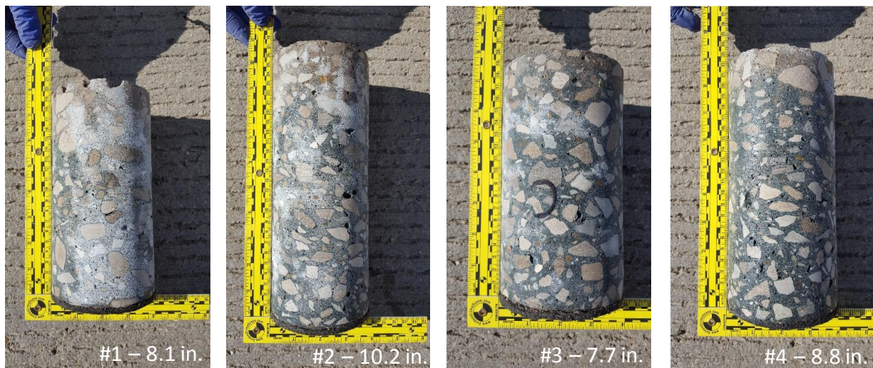
Thicknesses noted are thickness of PCC + fabric
