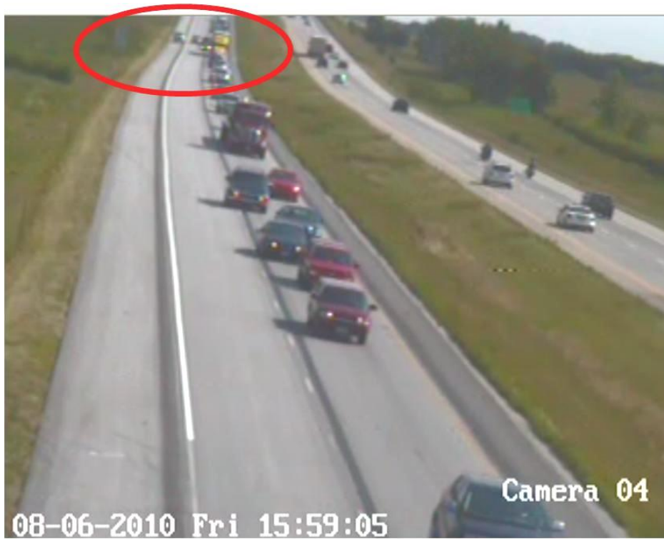
Figure 6.2. Lane straddling results in drivers passing on shoulder
