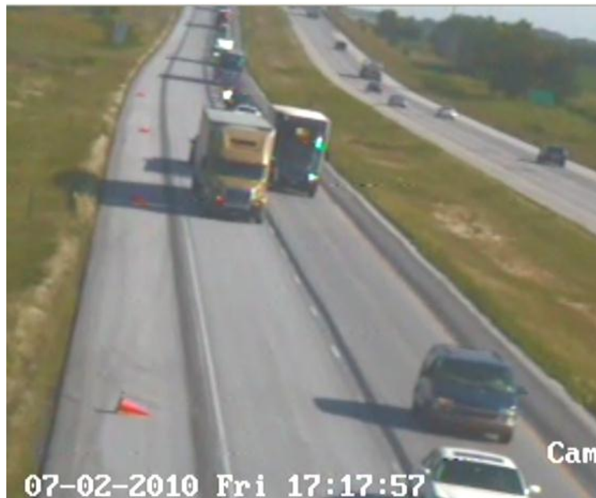
Figure 5.5. Lane-straddling vehicle driver creates large gap attempting to stay even with upstream vehicle to prevent passing
