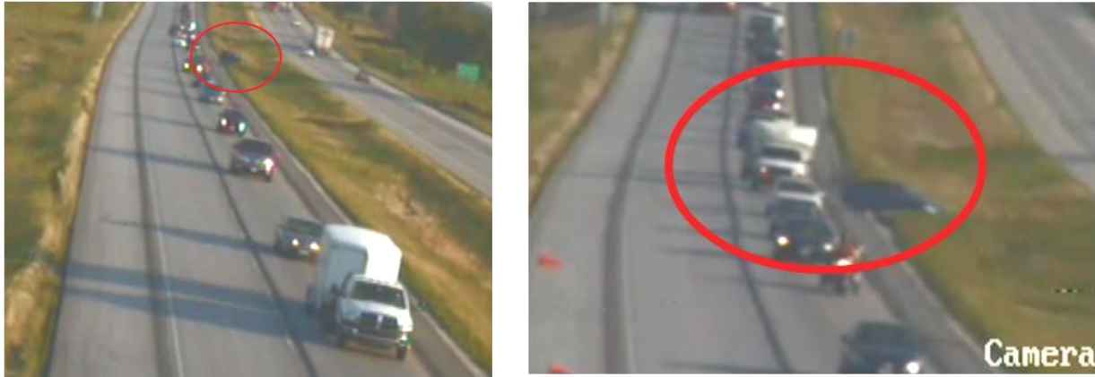
Figure 6.4. Vehicles turning around in the median
