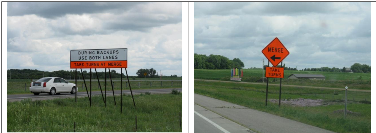
Figure 8.1. Use of late merge in Minnesota (Images courtesy of Willy Sorenson, Iowa DOT)
