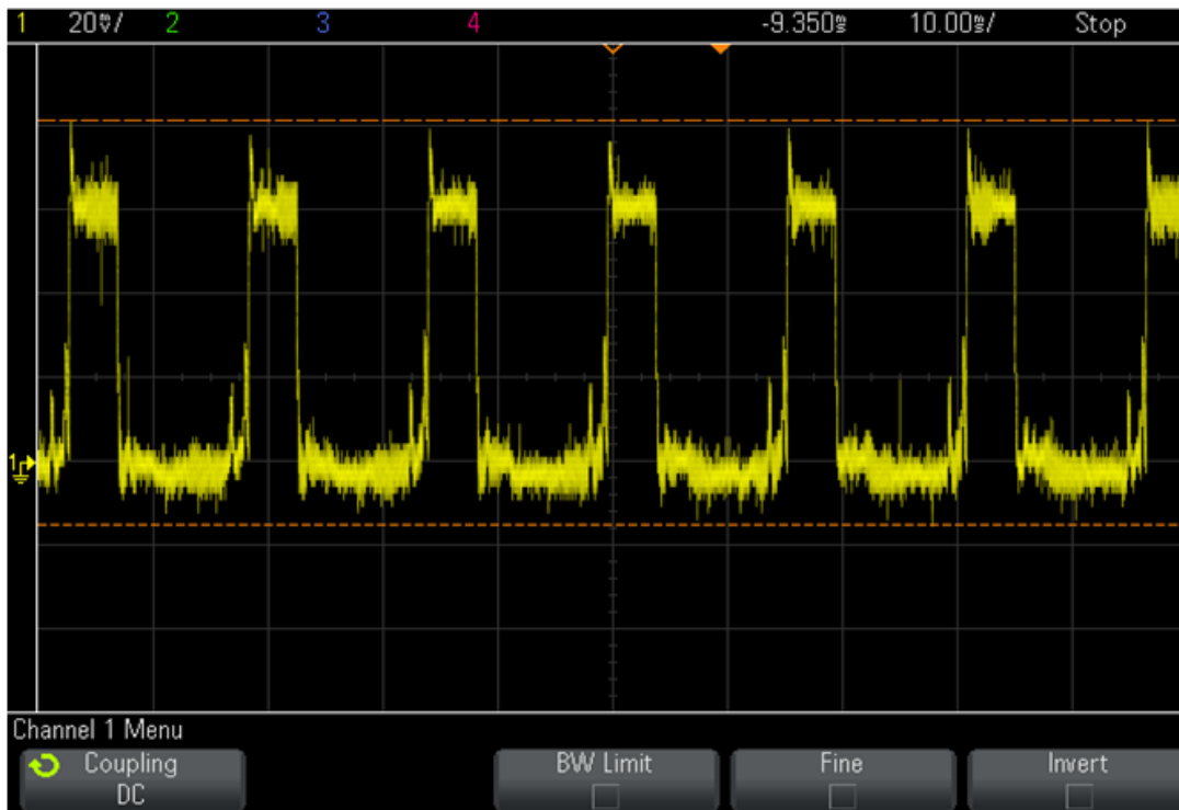
Figure 4. SG-Link node in synchronous burst mode
