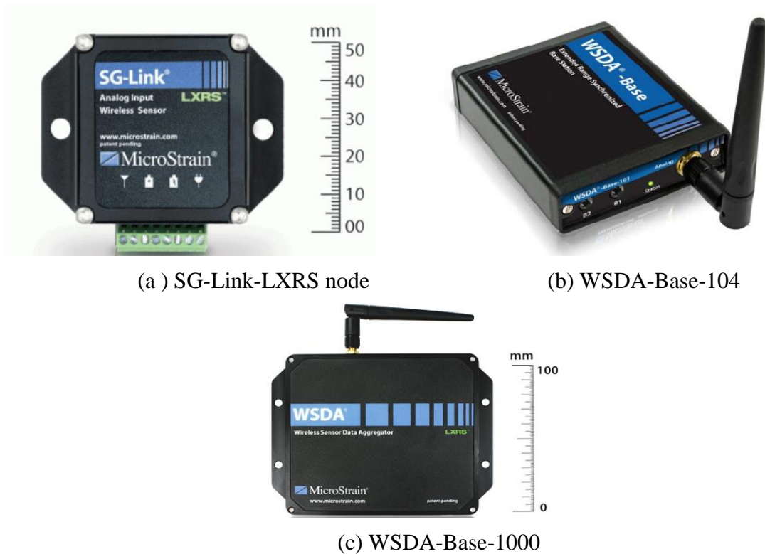
Figure 2. MicroStrain wireless sensor network platform
