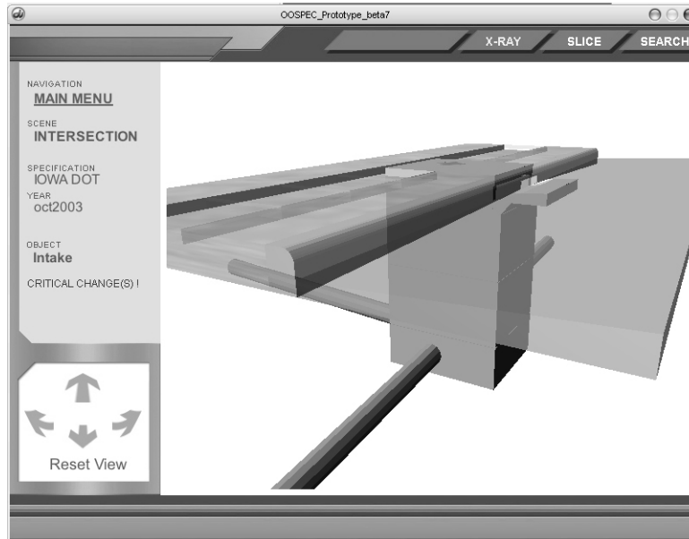
Figure 13. Object stage interface with the intake and sewer pipes
