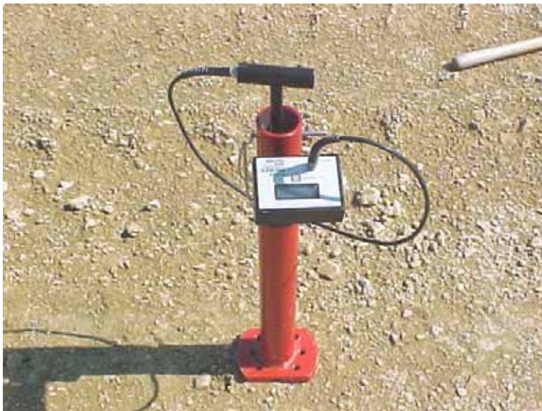
Figure 12. Clegg Impact Hammer
