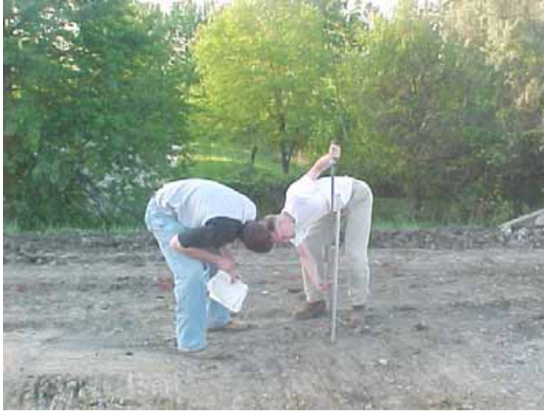
Figure 11. DCP testing on westbound entrance ramp of I-235 at 35th Street in West Des Moines, Iowa
