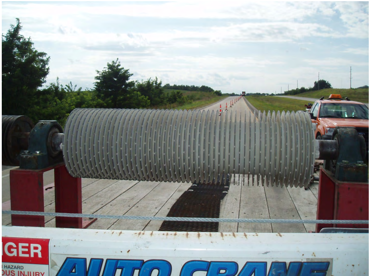
Figure 13. Grooving head (32 inches)
