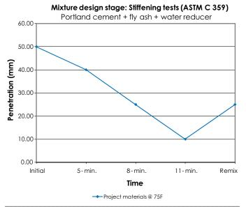
Figure 2. Example false set test results
