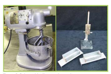
Figure 1. False set testing equipment
