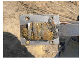
(c) high pressure shear plates after shearing
