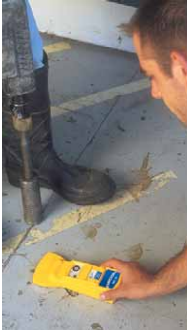
Figure 63. Zircon MT6 measures depth of metal to 6 inches +/- 1 inch
