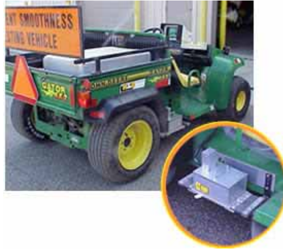
Figure 7. Ames Engineering, Inc., road profiling laser to test smoothness
