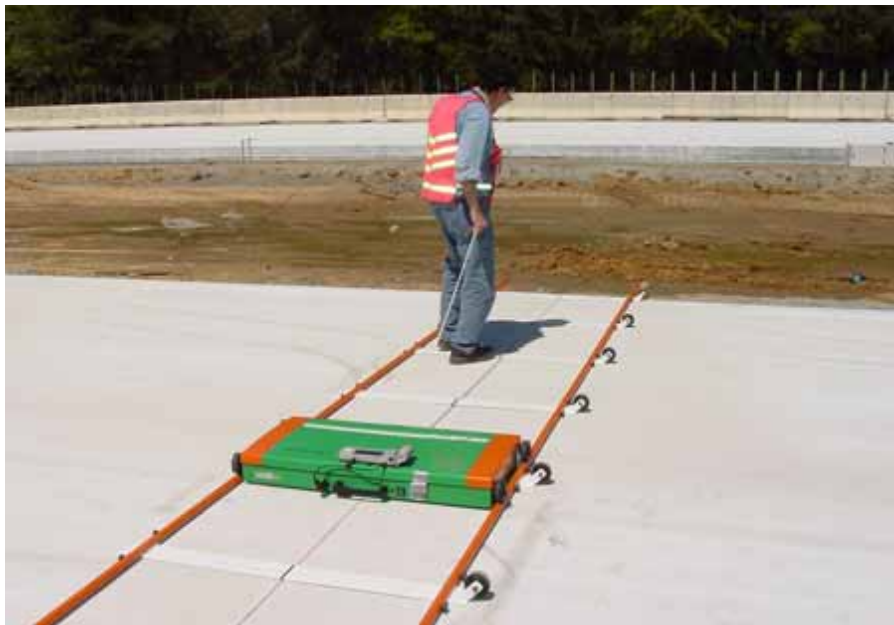
Figure 62. MIT Scan-2 uses magnetic pulses to measure the depth of dowel bars
