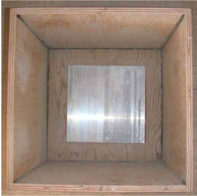
Figure 66. Test box with aluminum plate prior to pouring concrete
