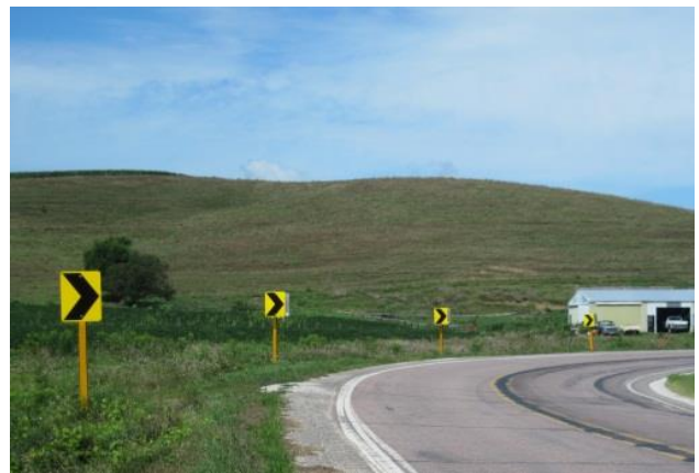
Figure 18. Delineator posts along a curve ( www.pexco.com/Pages/PexcoTrafficRDP.aspx )
