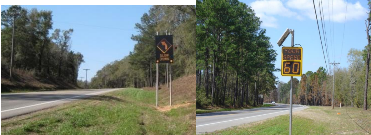
Figure 41. Dynamic speed feedback signs evaluated in six states
