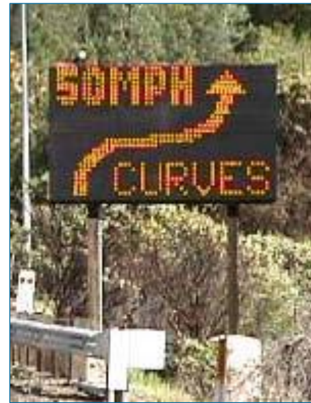
Figure 40. Speed warning sign in the Sacramento River Canyon (Tribbett et al. 2000)
