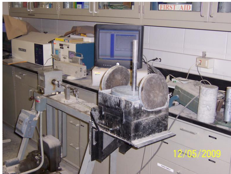
Figure 3-3. Direct shear test for concrete (all measurements between 15 - 30 min.)
