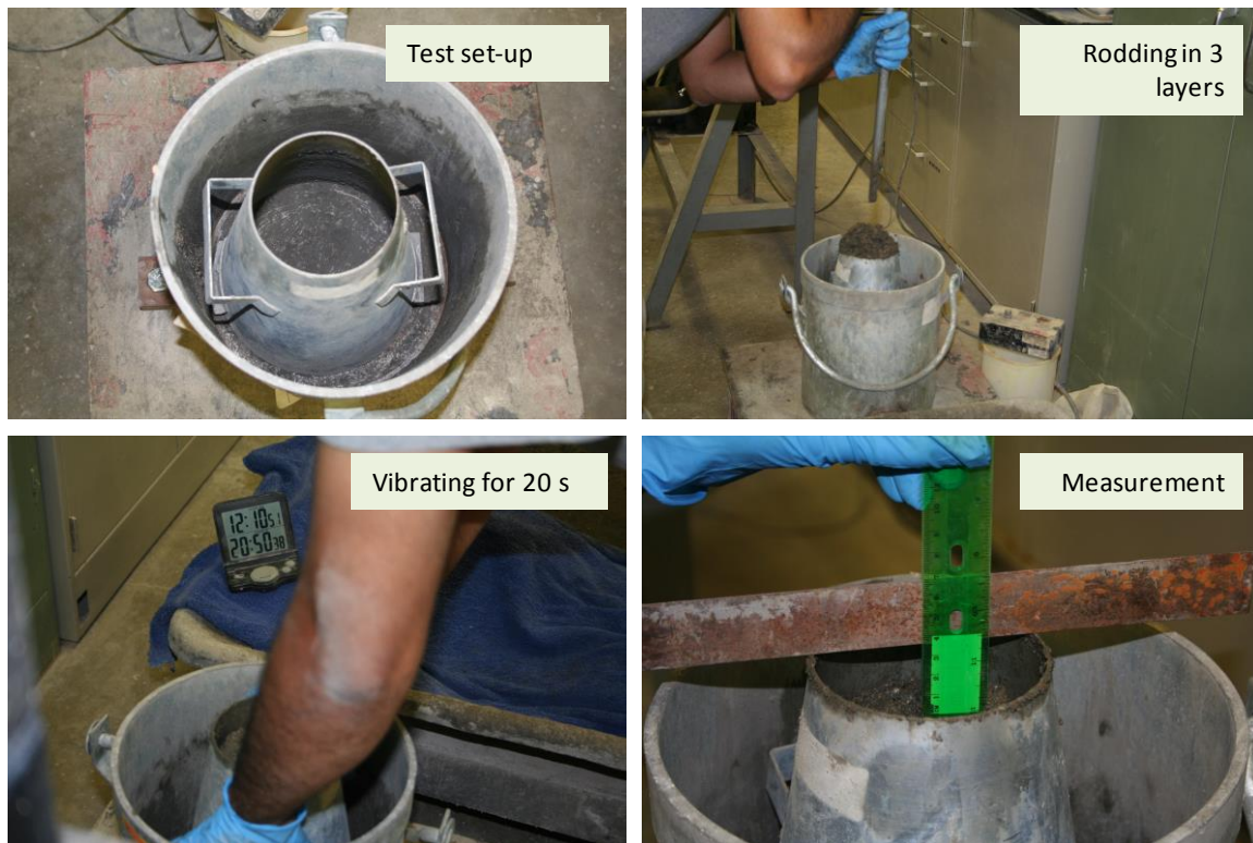
Figure 3-1. Test procedure for measuring consistency: CSV
