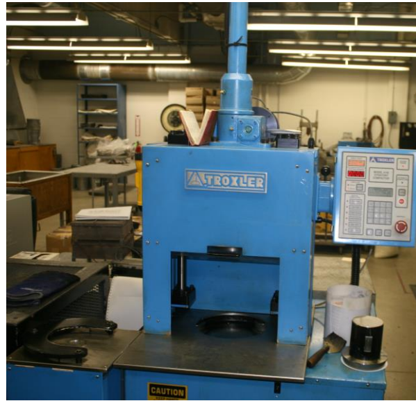
Figure 3-2. Gyratory compactor used in the work
