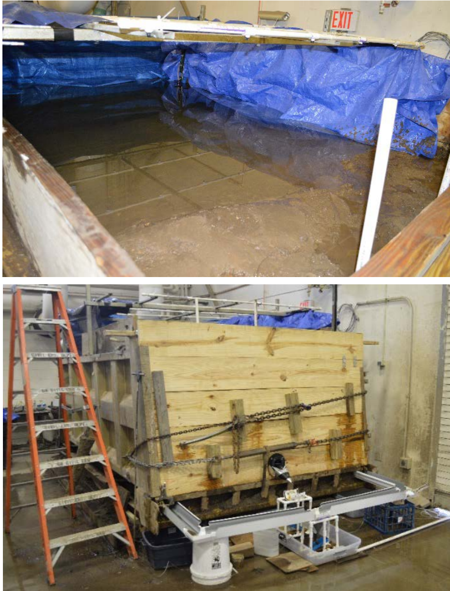
Figure 11. Water impounded behind wall as viewed from above model container (top) and front view of model retaining wall (bottom)
