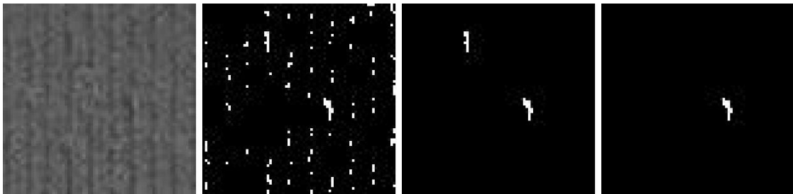
Figure 9. Example of non-crack pavement block with light longitudinal tined texture (from left to right): raw pavement block, local filtering, minor removal, and maximum extraction
