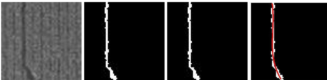
Figure 12. Example of polynomial fitting of continuous crack (left to right): raw crack block, maximum extraction, maximum expansion, and polynomial fitting
