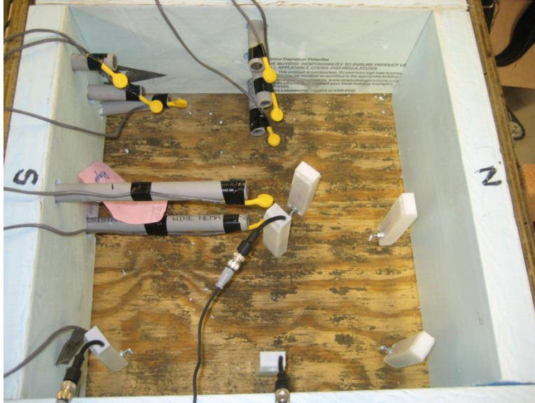
Figure 1. Temperature and humidity sensor layout
