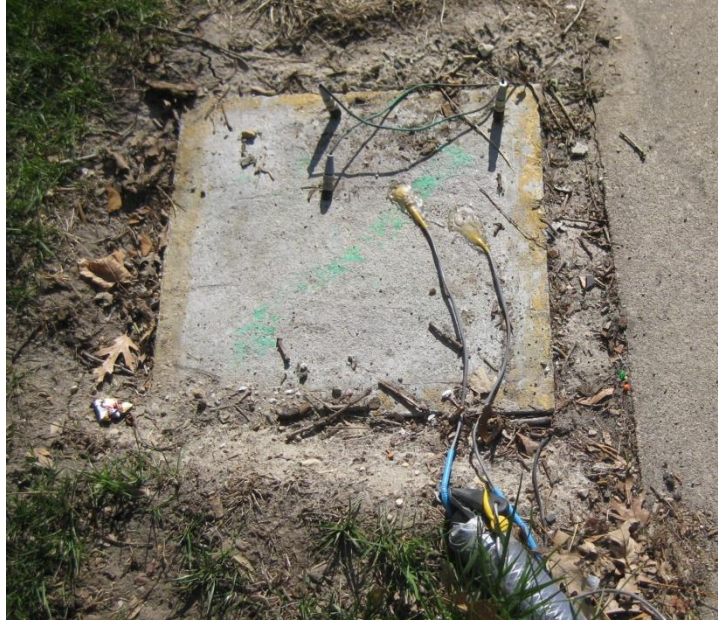
Figure 3. Instrumented slab buried in the ground next to a residential driveway
