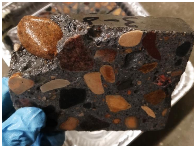
Figure 10. Laboratory sample exposed in 3% NaCl solution, showing cleanly exposed aggregate
