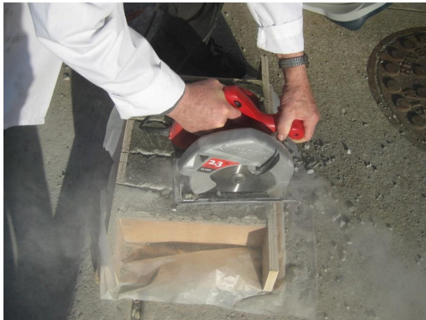
Figure 25. Saw cutting the test slab
