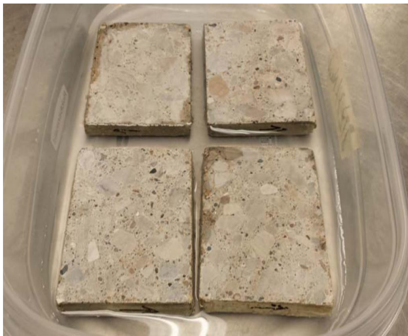
Figure 12. Samples partially immersed in liquid while stored at 40°F
