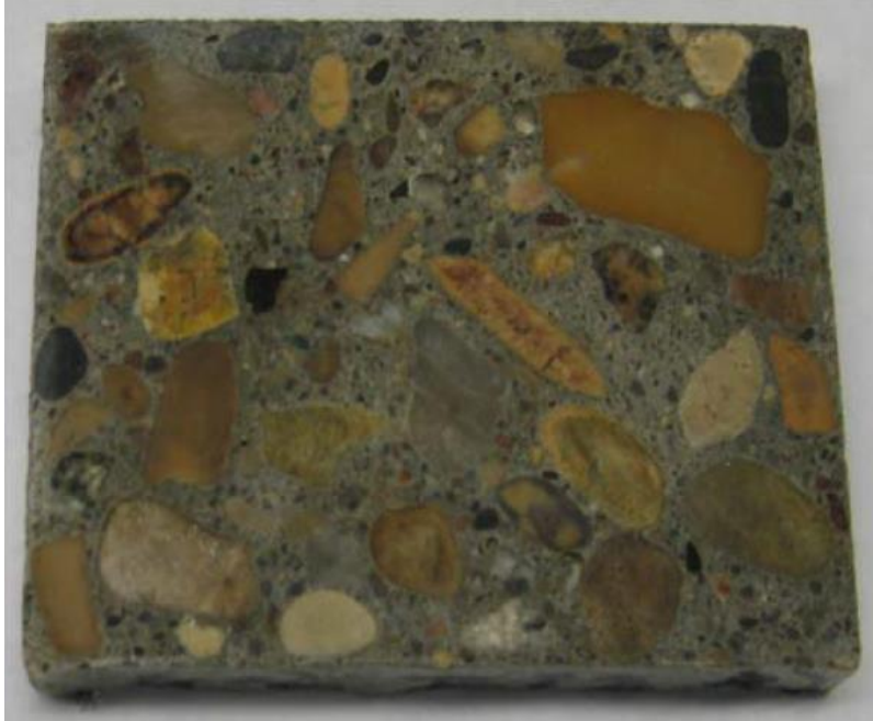
Figure 11. Saw cut slice sample with a thickness of 1/2 inch
