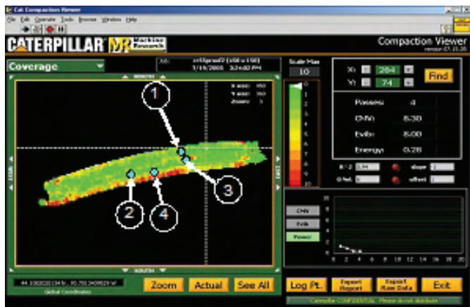
Field Study 1: Compaction monitor view at County 55 (viewing area 137 x 110 m) identified by DCP test locations
