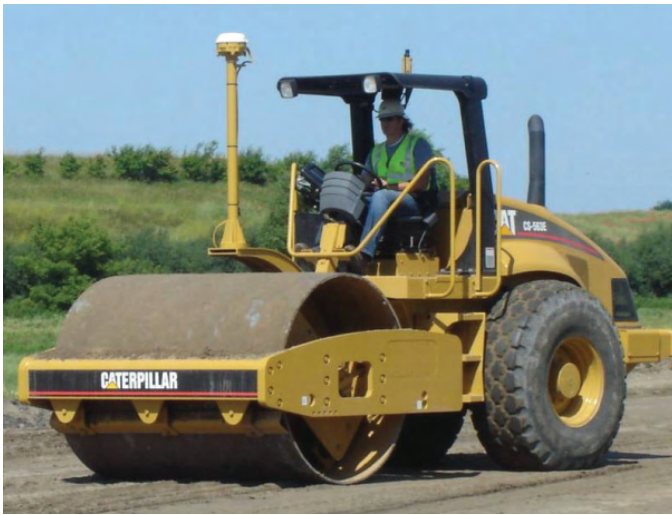
Caterpillar vibratory smooth drum roller with integrated CMV and MDP technology: Field Study 1
