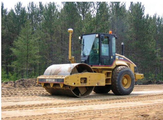
Caterpillar vibratory smooth drum roller with integrated CMV technology: Field Study 3
