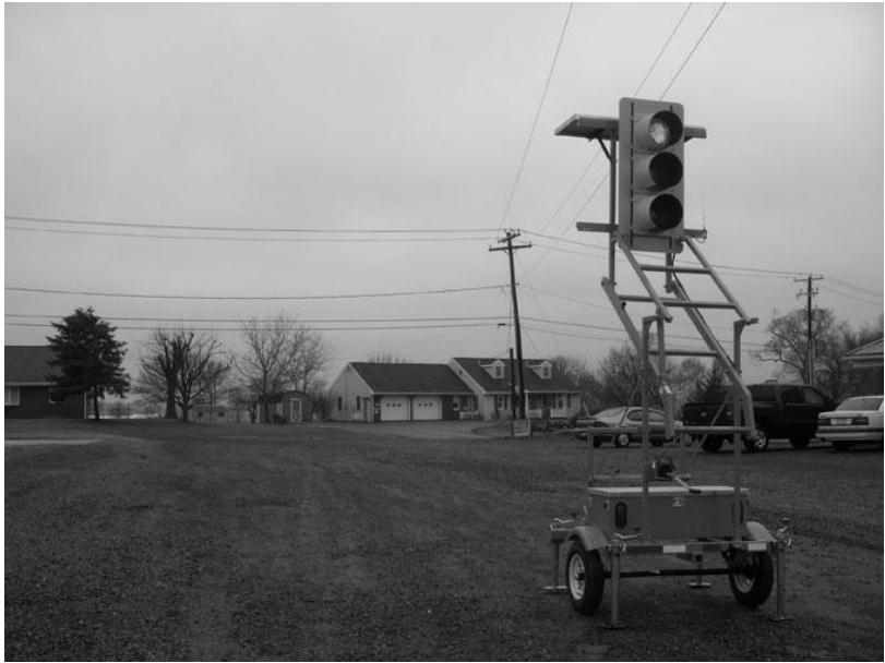
Figure C.2. Temporary signal lighting
