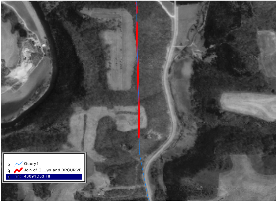
Figure 4 Deviation of Network Maps from the aerial photos (in very rare cases)
