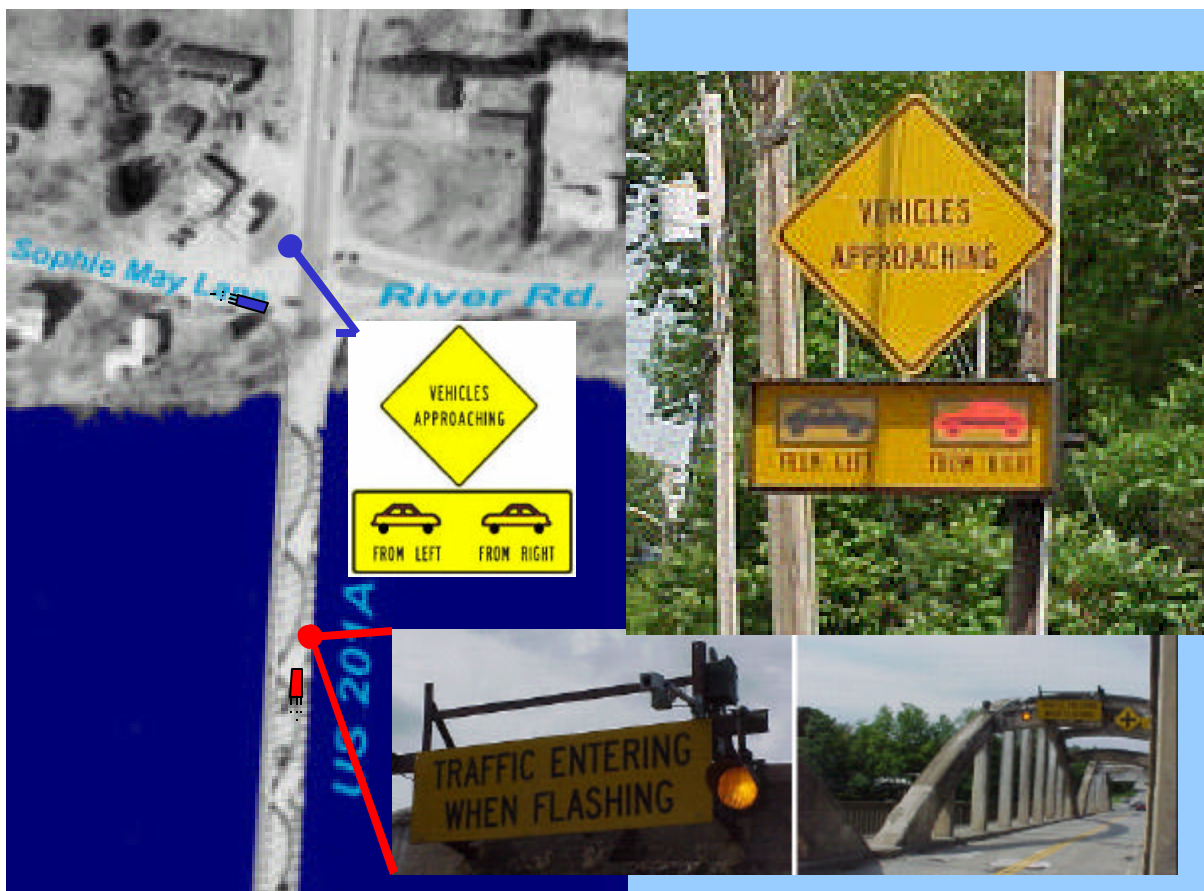
Figure 2.16. Layout of the conflicting traffic warning system used in Maine (10)
