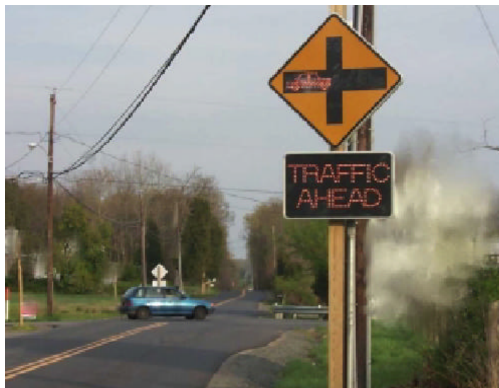
Figure 2.15. Intersection collision warning system major approach (36)
