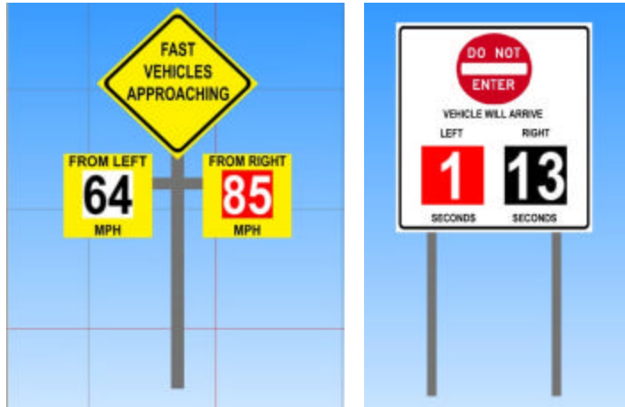
Figure 2.18. Proposed designs for dynamic signs (Source: ITS Institute, University of Minnesota)
