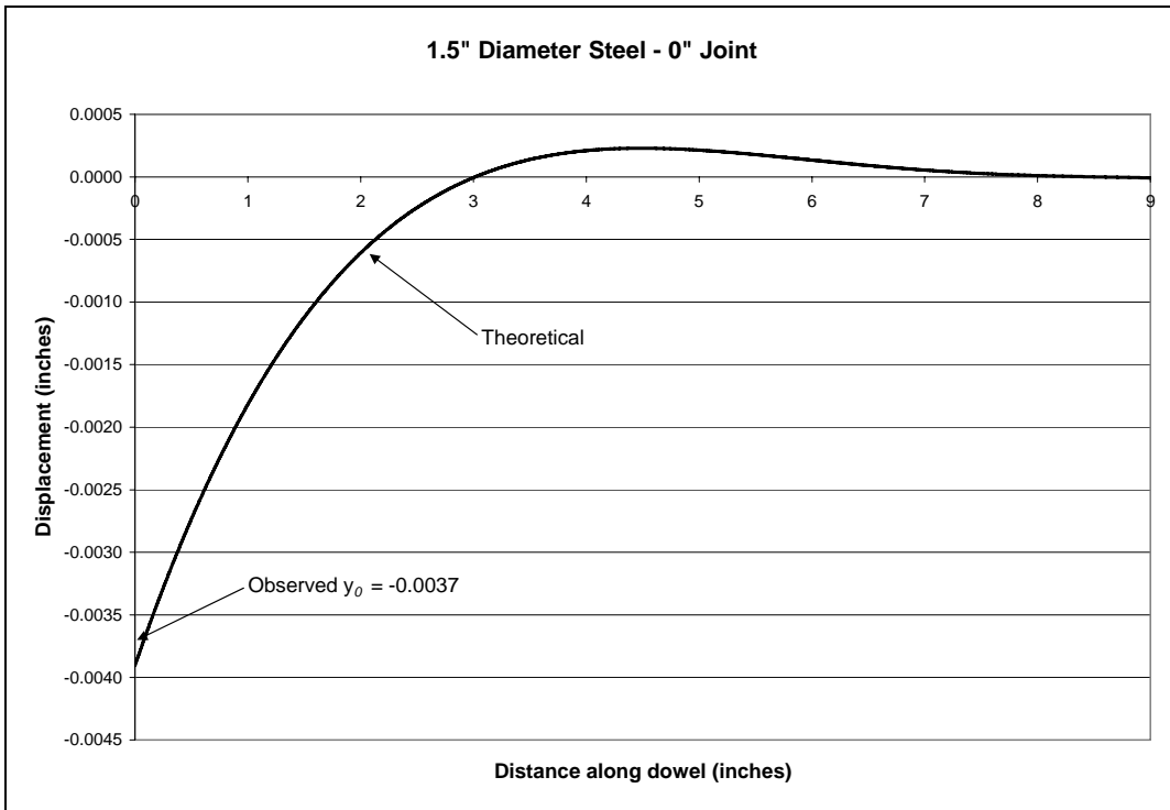
Figure C.1. Theoretical displacement of round steel dowel, 0-inch joint
