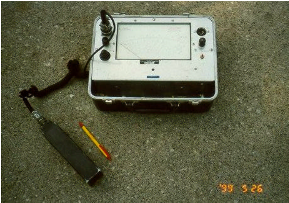
FIGURE 4.1 Pachometer Used to Locate Reinforcing Steel in a Bridge Deck
