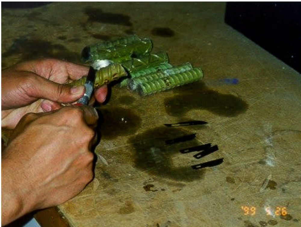
FIGURE 4.10 Epoxy Coating Bond Test
