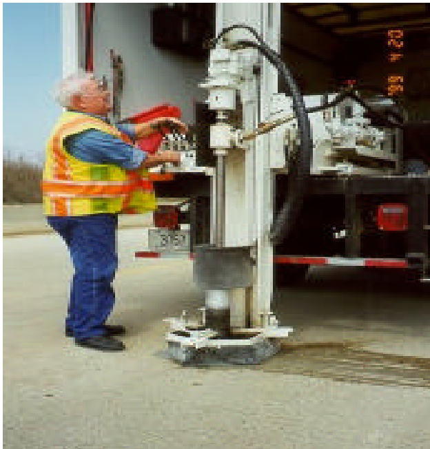
FIGURE 4.2 The Setup of the Coring Process
