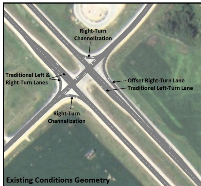
Figure 1. Existing conditions geometry
