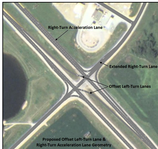
Figure 3. Offset left turn lanes and right turn acceleration lane geometry
