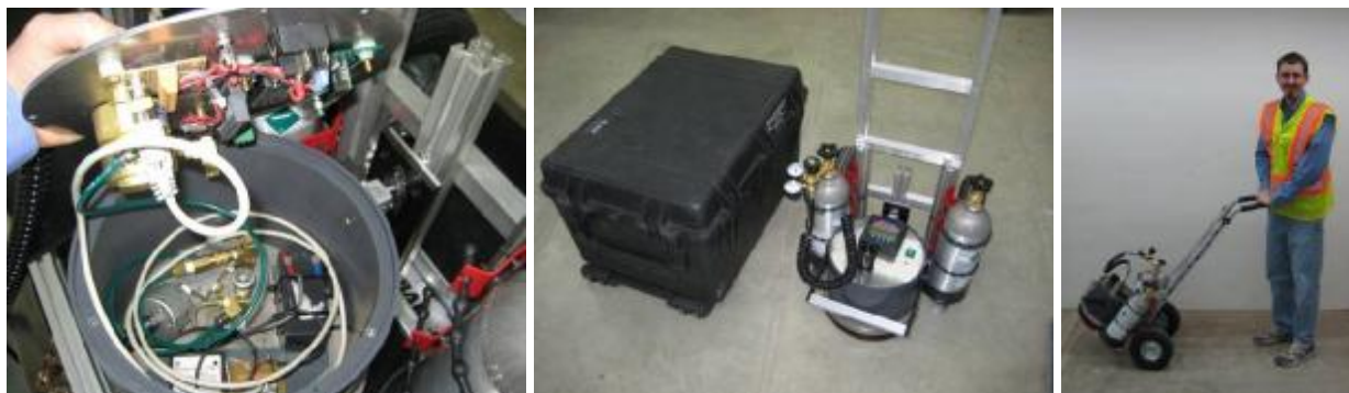
FIGURE 3 Internal ruggedized sensor components, regulator, and circuit board for digital display (left); pelican case for shipping and handling (middle); wheel cart pick-up device with two aluminum CO 2 cans (right)
