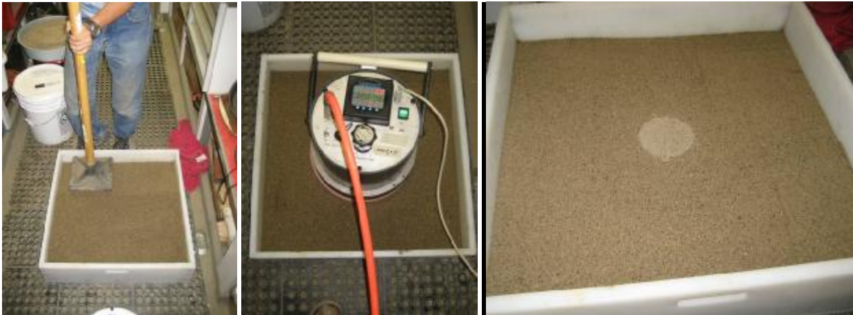
FIGURE 13 Pictures showing compaction (left) and testing (middle) process on materials at different degrees of saturation and a picture showing dry material at the surface that is in contact with the orifice outlet after testing with GPT device (right)
