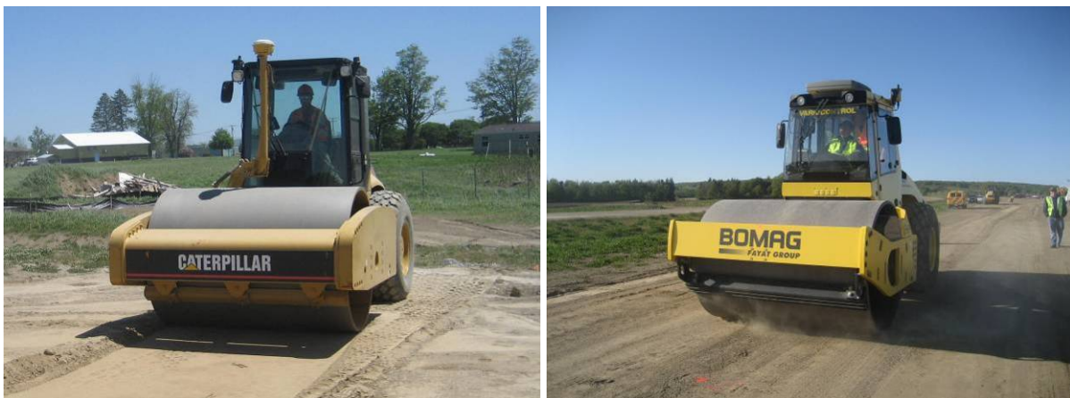
Figure 1. Caterpillar CS683 (left) and Bomag BW213-H (right) vibratory smooth drum IC rollers
