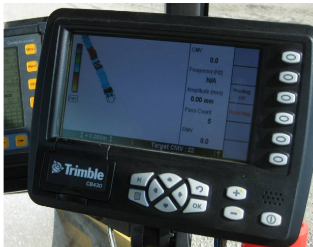
Figure 15. Trimble CB430 on-board display unit with roller-integrated CMV measurement system
