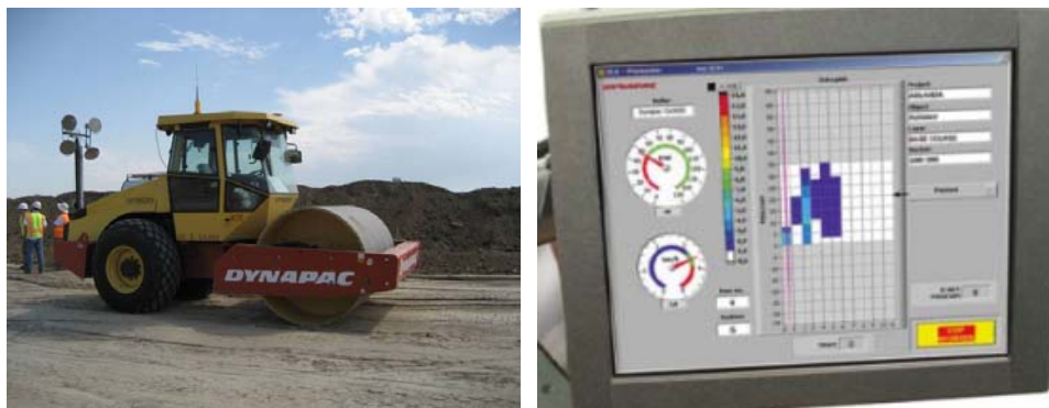
Figure 13. Dynapac rollers (padfoot and smooth drum) equipped with roller-integrated CMV measurement system and on-board display unit with DCA ® software
