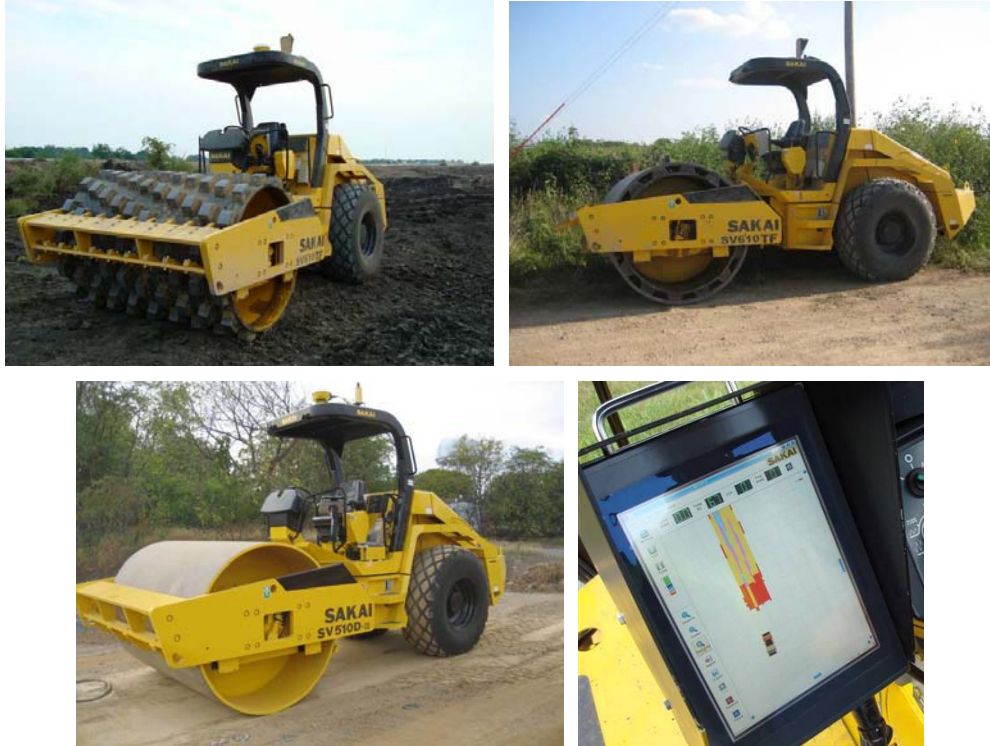
Figure 14. Sakai rollers (padfoot and smooth drum) equipped with roller-integrated CCV measurement system and on-board display unit with Aithon-MT ® software
