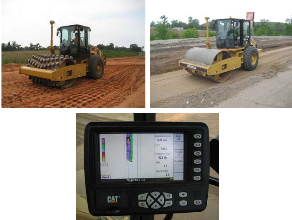
Figure 12. Caterpillar rollers (padfoot and smooth drum) equipped with roller-integrated MDP and CMV measurement systems on-board display unit with AcuGrade ® software
