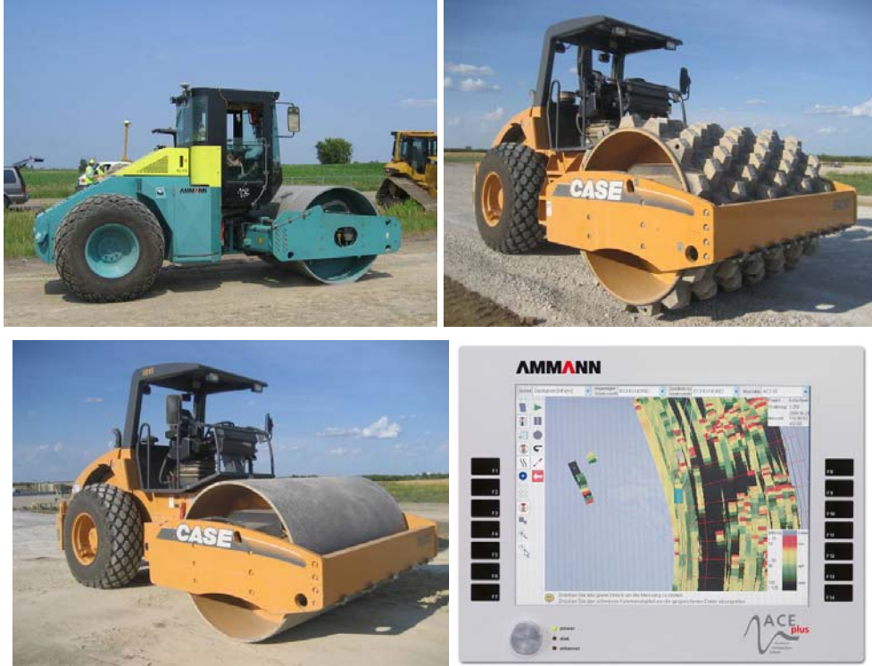
Figure 10. Ammann and Case rollers (padfoot and smooth drum) equipped with roller-integrated k_s measurement system on-board display units with ACE-Plus ® software
