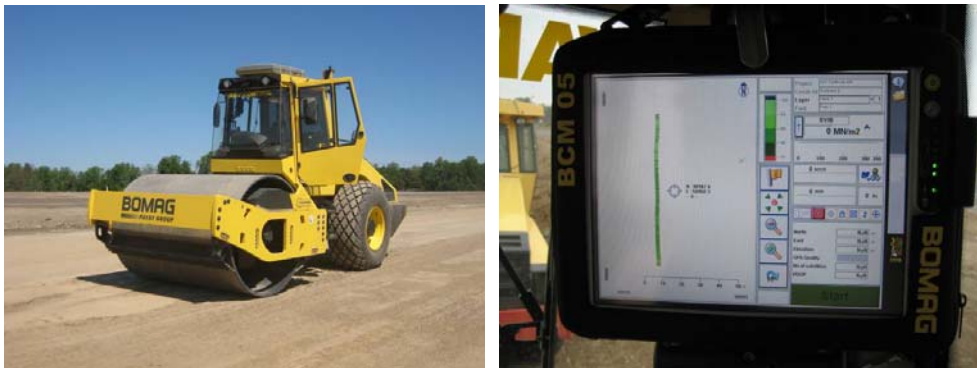
Figure 11. BOMAG rollers (padfoot and smooth drum) equipped with roller-integrated E_{VIB} measurement system on-board display units with BCM-05 ® software
