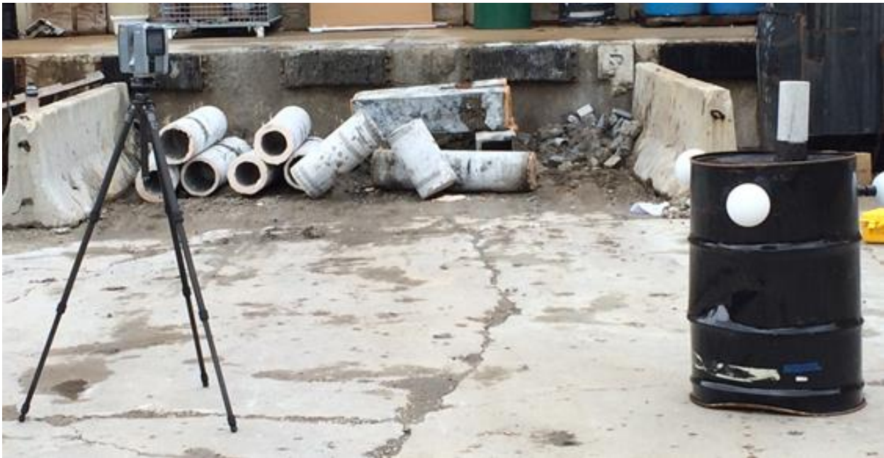
Figure 9. Laser scanning of a concrete block
