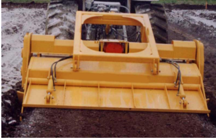
Figure 8. Type MGM 250 soil mixer (Gutzwiller 2006)
