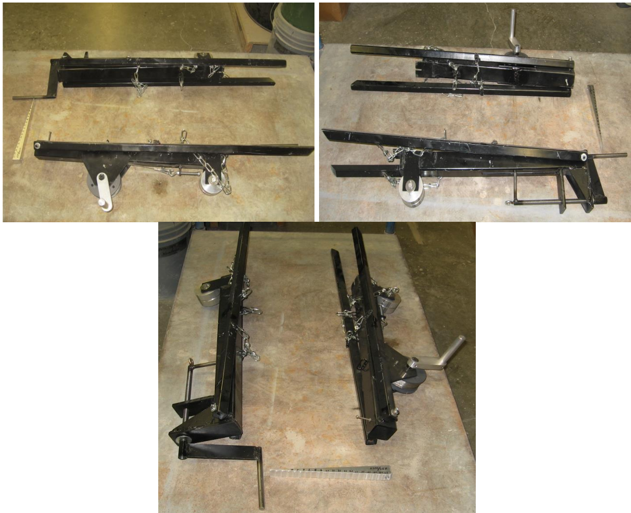
Figure 25. First generation of ISU curling and warping device: front view (top left), back view (top right), and side view from head (bottom)
