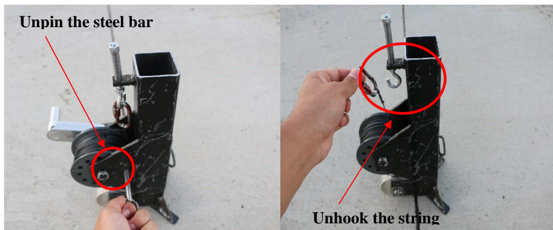
Figure C.2. Unpin the bar and unhook the string
