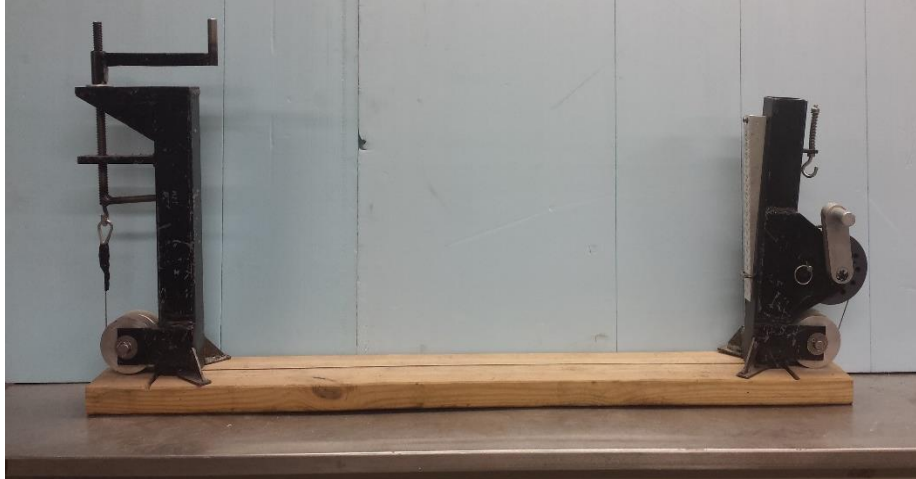
Figure 28. Overview of second generation of ISU curling and warping measurement device
