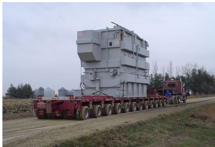
Electrical transformer en route to a wind energy tower contributing to rutting (Photo courtesy of Mitchell County)
