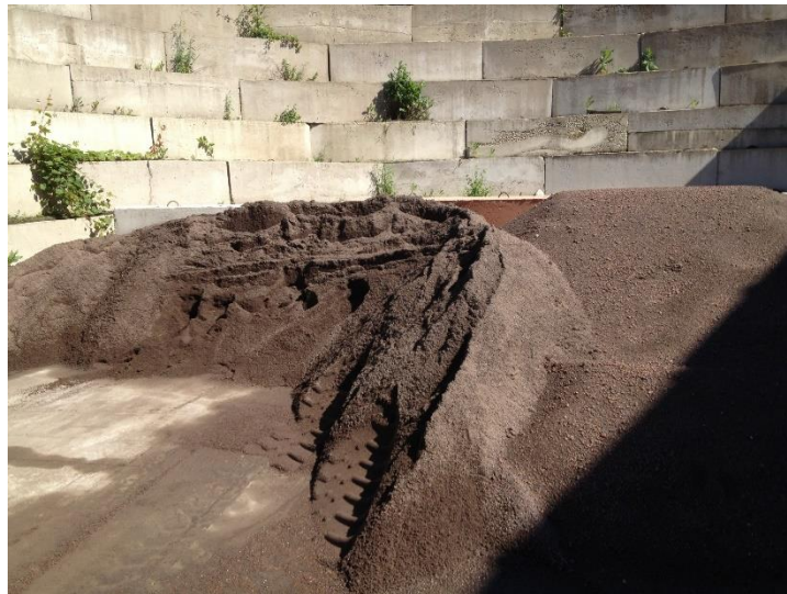
Figure 7. LWFA pile before mixing at central mix plant
