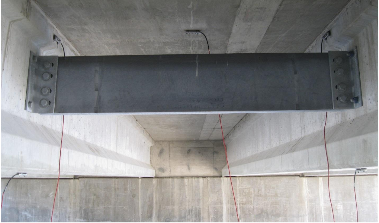
Figure 14. Typical instrumentation setup for testing of LWFA bridge
