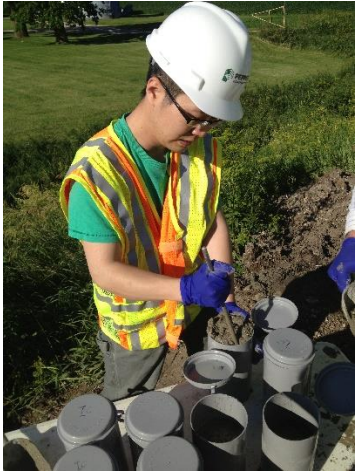
Figure 10. Concrete sample preparation
