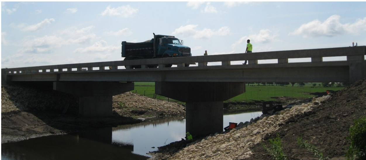
Figure 12. Live load testing of LWFA bridge, 2013
