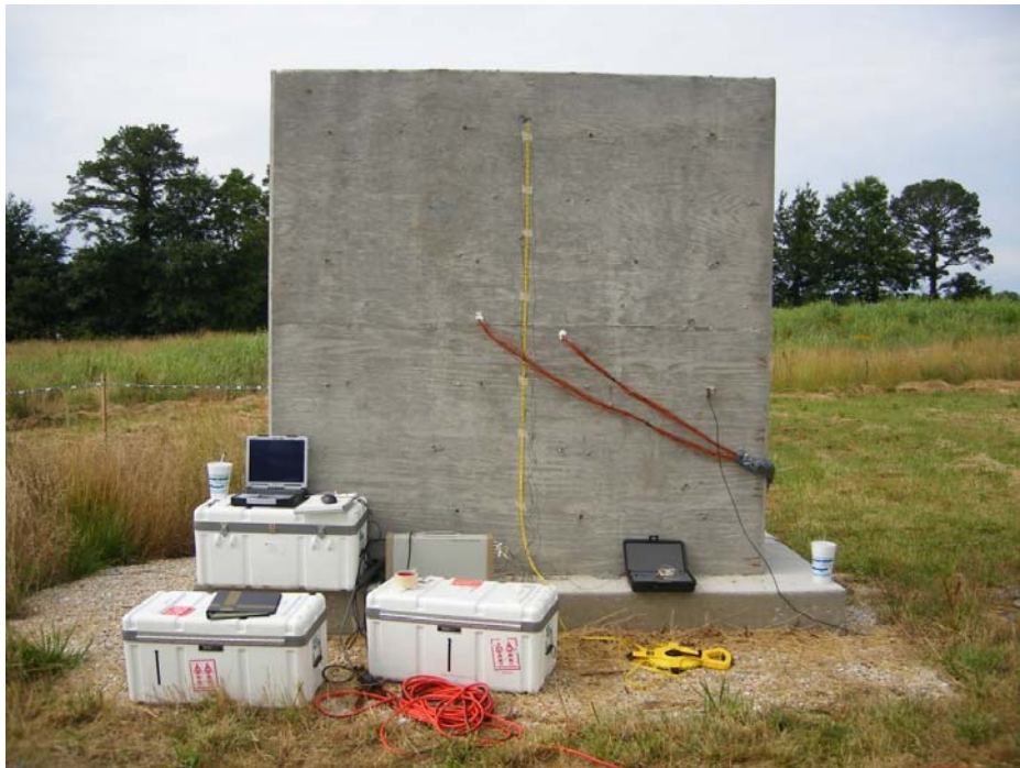
Figure 24. Concrete block with subsurface defects at the Midway site
