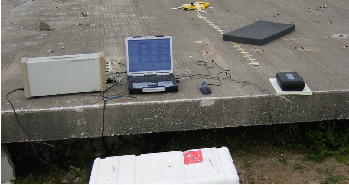
Figure 7. Experimental arrangement used to collect measurements at the RTF bridge deck site
