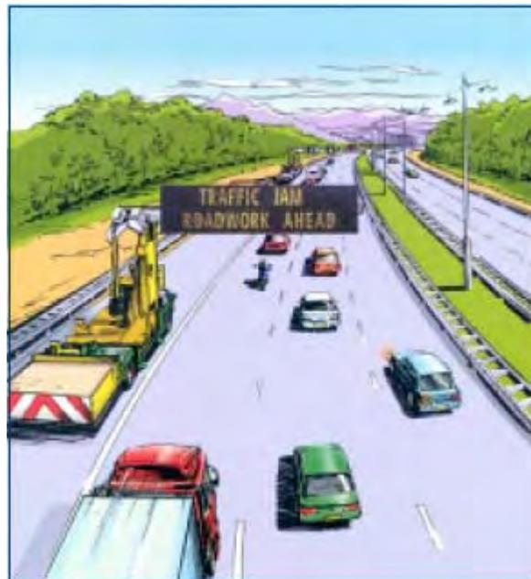
**Figure 2. Portable sign gantries in the Netherlands (Steinke et al. 2000)**
