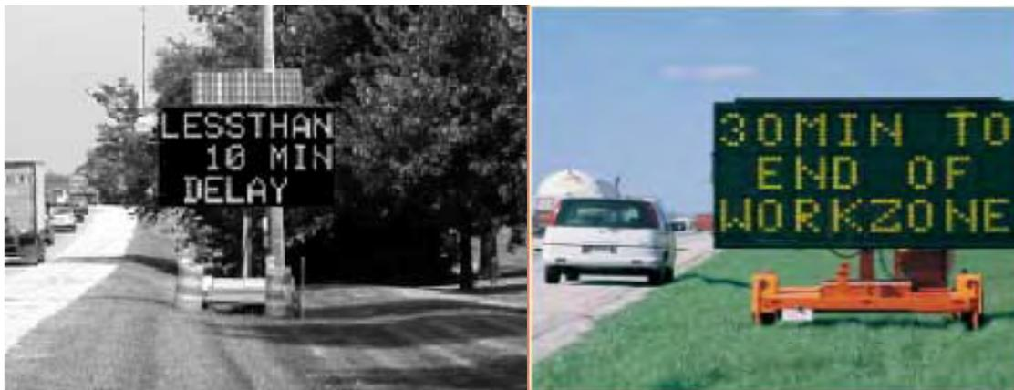
**Figure 3. Examples of delay and travel time estimation system displays (FHWA 2001b)**
