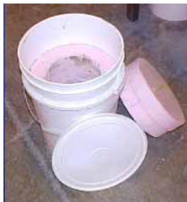
Figure C3. Lafarge basket test setup
