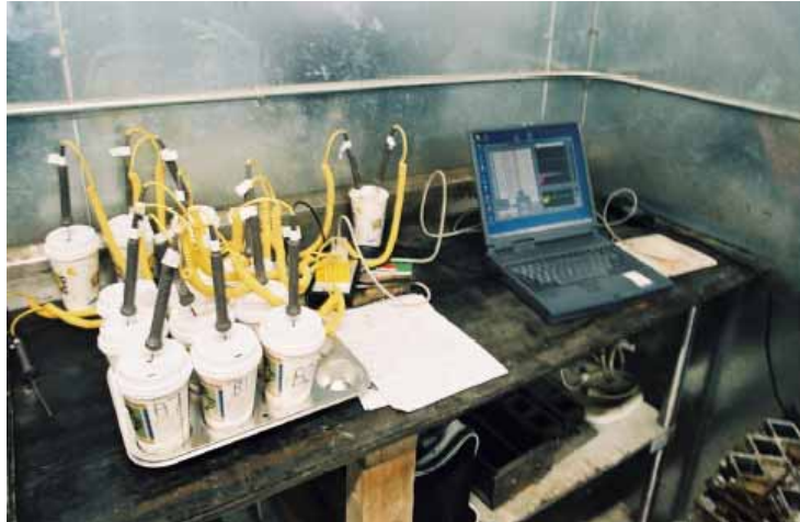
Figure C2. Coffee cup test setup (Gary Knight, Holcim, 10/1/2004 TWP meeting)
