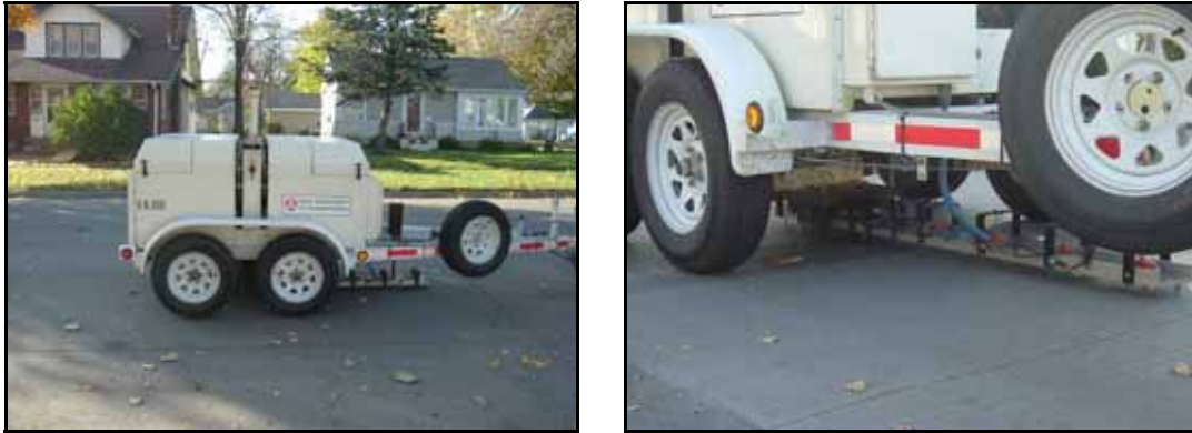
Figure 51. Falling weight deflectometer
