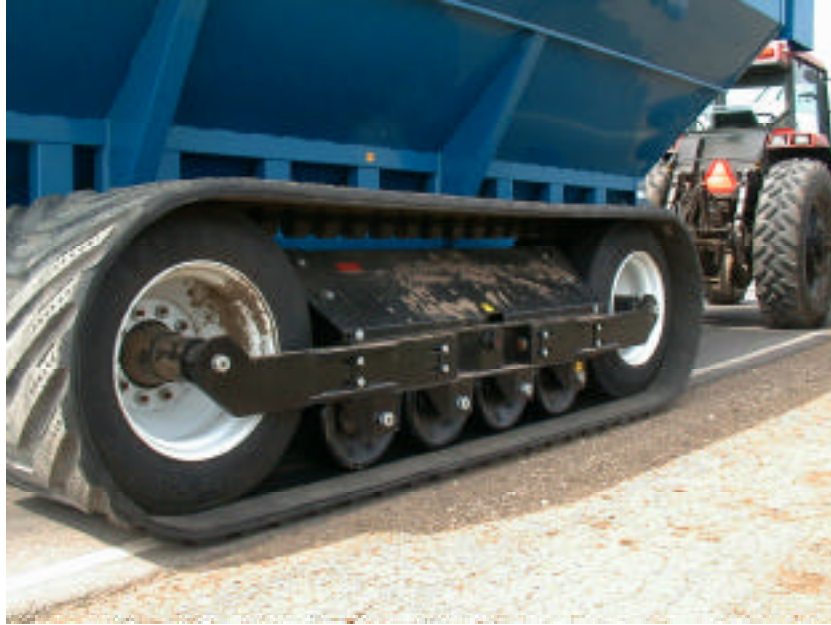
FIGURE 1 KINZE 1040 tracked wagon used in pavement testing.
