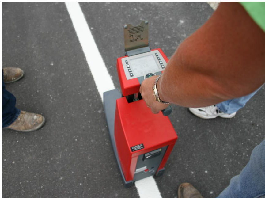
Figure 3. Measuring retroreflectivity using the a handheld device (LTL-X)
