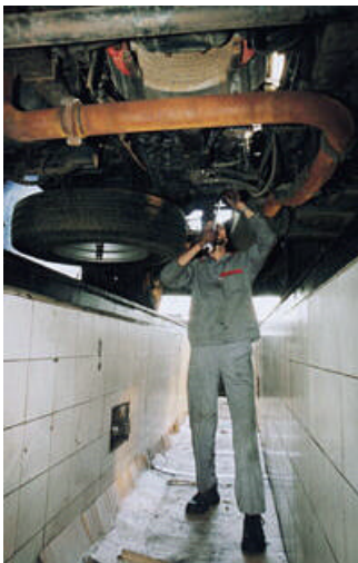
Fig.3. Underground pits system
