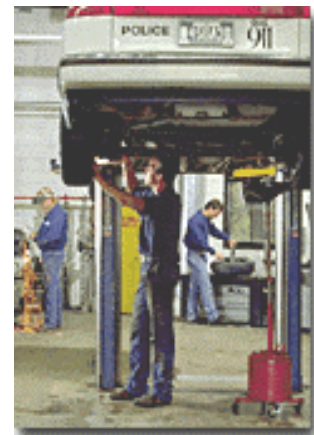
Fig. 2. Vehicle lift system
