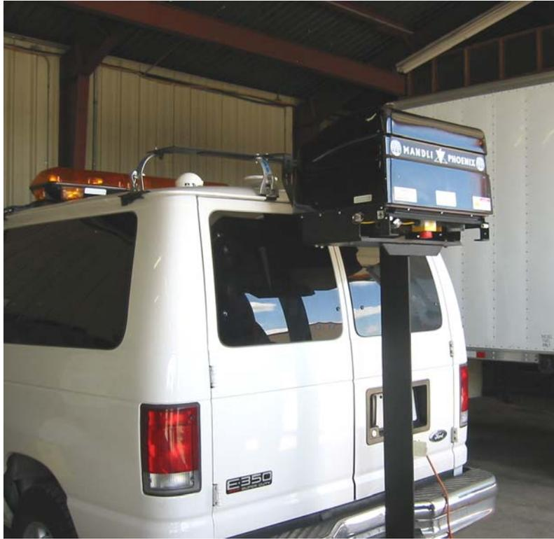
**Figure 2. PPS device mounted on the Iowa DOT video log van**
