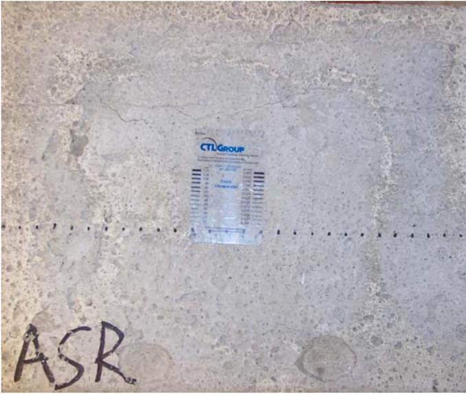
Figure 8. Surface cracking on the specimen containing ASR-reactive aggregate
