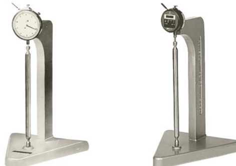
(e) Length Comparator (with Mechanical Indicator HM-250; with Digital Indicator HM-250D) (Gilson and Humboldt)
