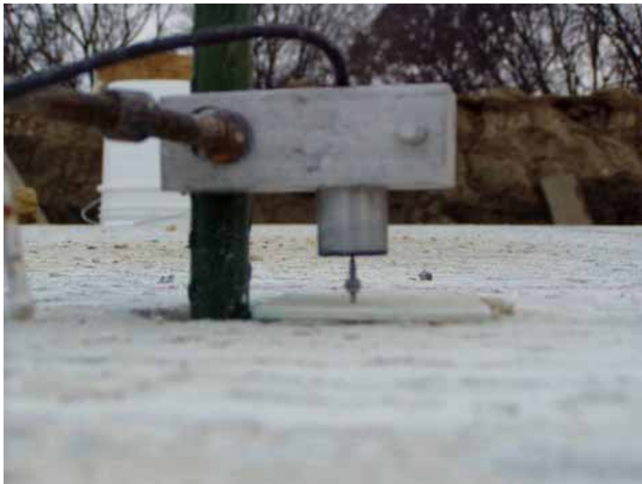
Figure 12. LVDT installation (Iowa State University)
