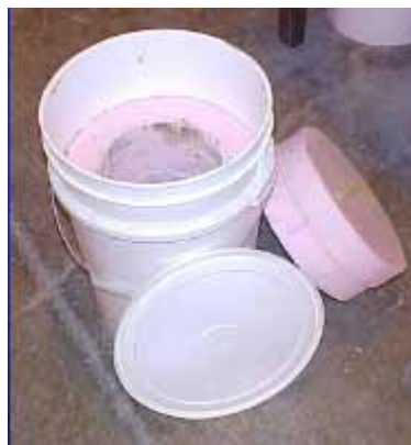
Figure C3. Lafarge basket test setup
