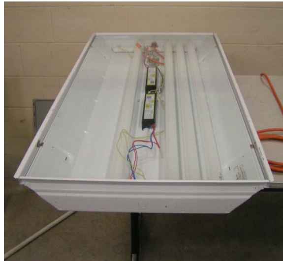
Figure 3.4. Setup for exposing circuit boards
