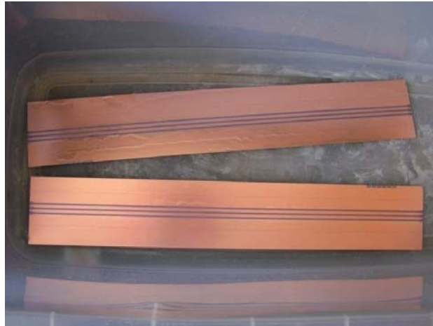
Figure 3.6. Exposed boards in the chemical bath
