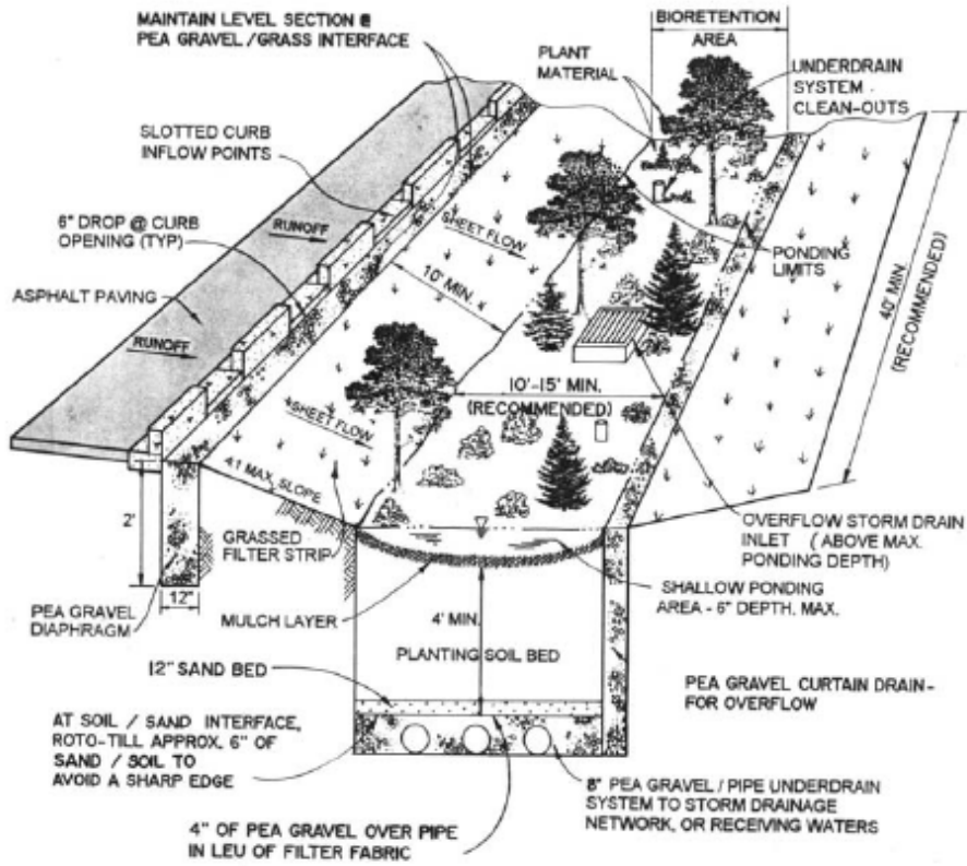
Figure 2: Bioretention system components
