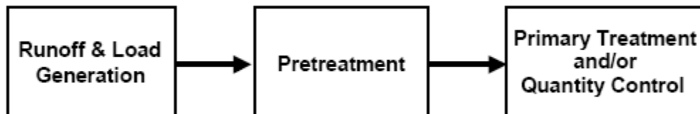
Figure 7: Generalized stormwater treatment train
