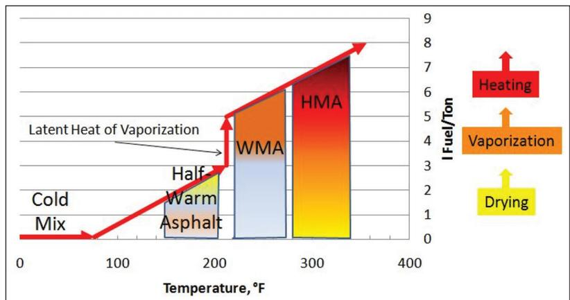
Warm-mix asphalt temperatures range from 30 to 100 degrees Fahrenheit cooler than hot-mix asphalt (and stay above 212 degrees) (Prowell 2007) <http://international.fhwa.dot.gov/pubs/wma/summary.cfm>
