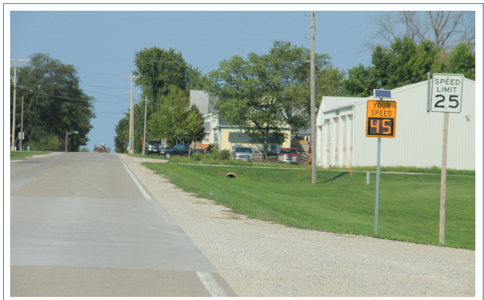
DSFS installed at Rowley east community entrance
