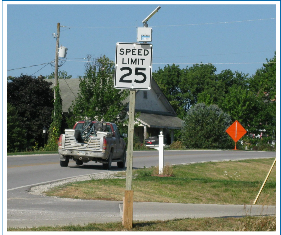
Radar-activated LED speed limit sign
