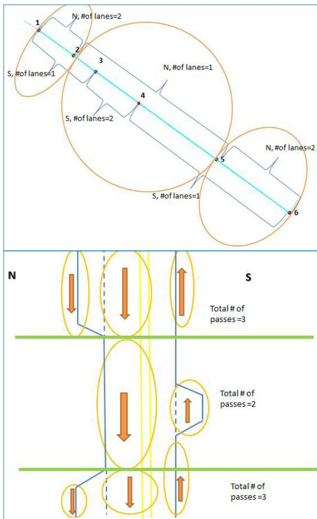
*Example of “difficult” segment for which number of passes and end/start points are different (top) and how the segment looks with the different number of passes for striping operations (bottom)*
