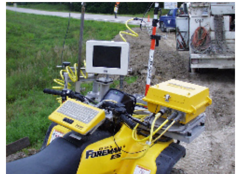
GPS installed on the all-terrain vehicle for staking and other survey work
