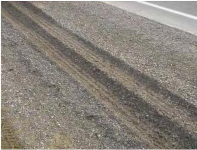
*Performance of the fly ash–stabilized shoulder section after seven months: stabilized section (top) and control section (bottom)*
