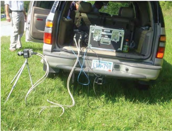
Monitoring tire-aggregate interaction using stationary high-speed camera
