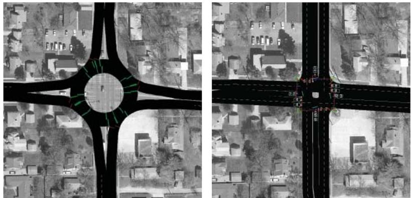
*Models of two alternative improvement projects proposed for an intersection in Ames, Iowa: roundabout (left) and turning lanes (right)*
