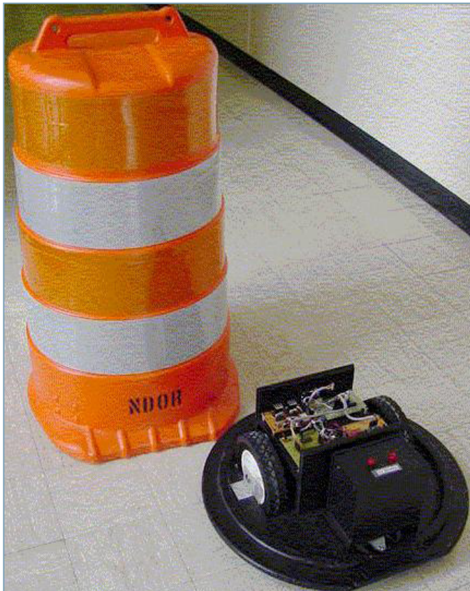
Robotic safety barrels show promise in reducing the number of workers and vehicles required to close lanes and move lane closures at the same pace as the mobile operations
