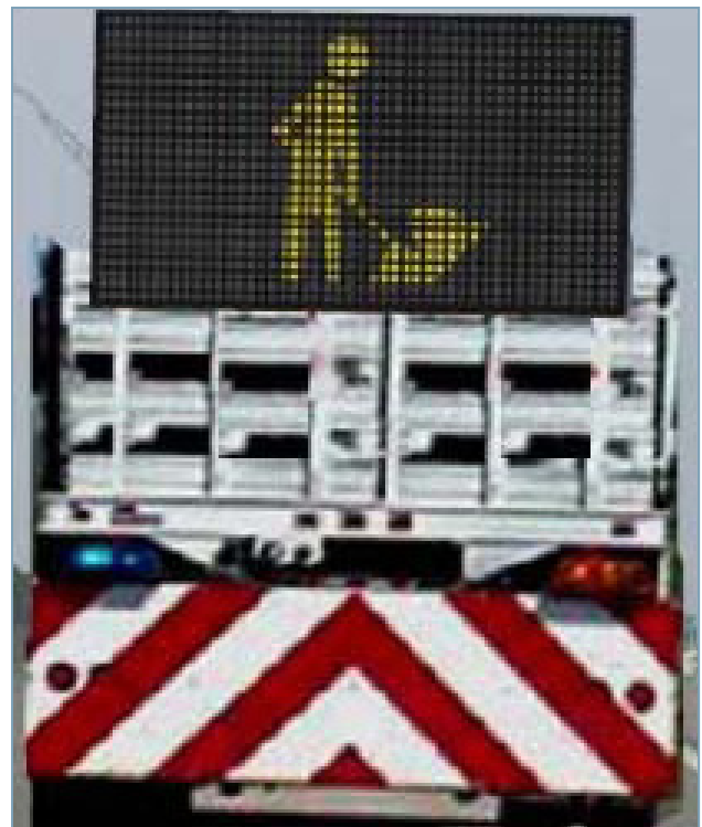
Truck-mounted changeable signs enable message delivery close to the actual work site (photo Texas A&M University-Kingsville)
